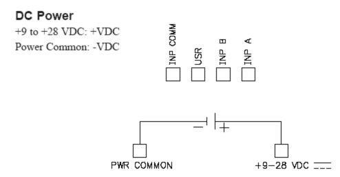
**FM-CNTUD-DCTBC** - Digital Counter, Scaleable directional up/down counts, Face Mount, DC Powered, terminal block connections.
