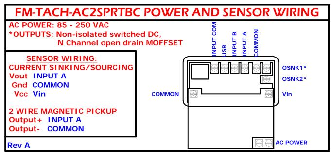
**FM-TACH-AC2SPRTBC** - Digital Dual Output Tachometer, Face Mount, AC Powered, terminal block connections, dual sinking open collector outputs
