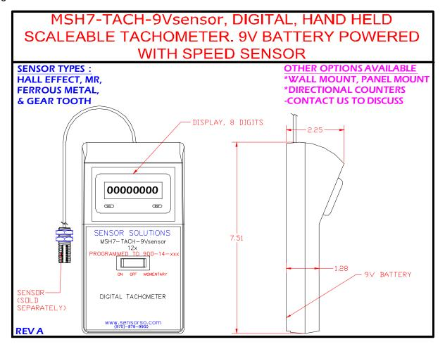
Our Digital Hand Held Tachometer provides a rate measurement that is determined by the frequency at which an attached digital sensor output is triggering\*. The meter can be paired with Hall Effect, Magnetoresistive, Gear Tooth, and Ferrous Metal detection sensors. The displayed rate is scaled based upon customer requirements.
